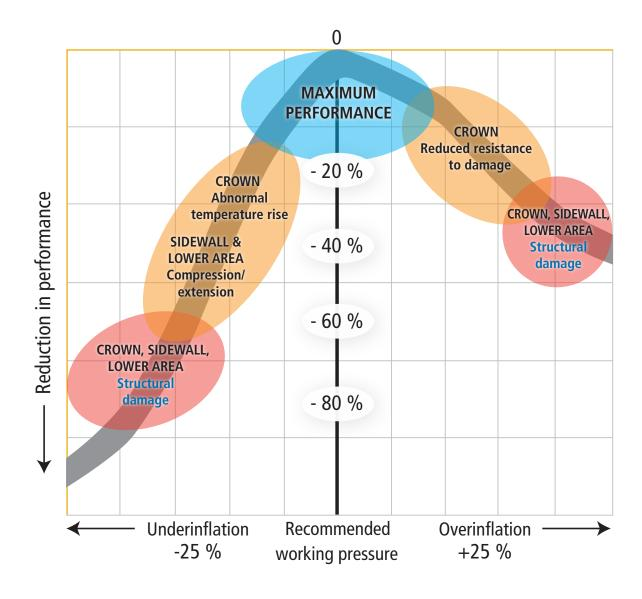
where incorrect front and rear balances can cause tipping. The operating pressure can be given by your tire manufacturer rep, or by an authorized professional who will consider tire usage criteria (type of machinery, type of soil, length of cycles, materials transported, loads, etc.).
